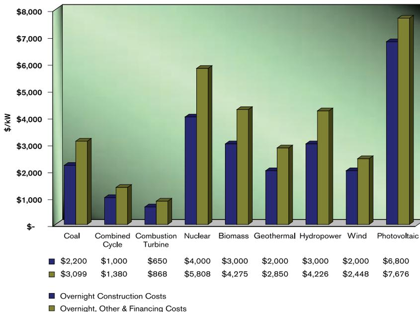
Figure 2: Overnight vs Total Construction Costs to Build
